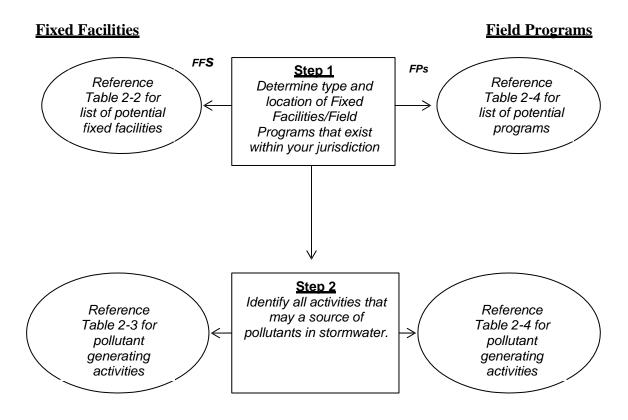
Figure 2-1 Inventory Process for Fixed Facilities and Field Programs
