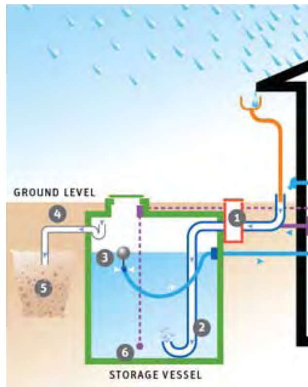
Figure 7.16 Typical cistern components
